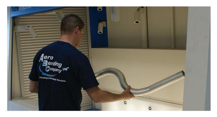
One of Aero Bending's staff of eight bending machine operators places a bent tube onto the measurement bed of a TubeInspect optical measurement system from Aicon 3D. Because it's a camera-based system, it instantly measures the entire tube length to create a 3-D image of it.
