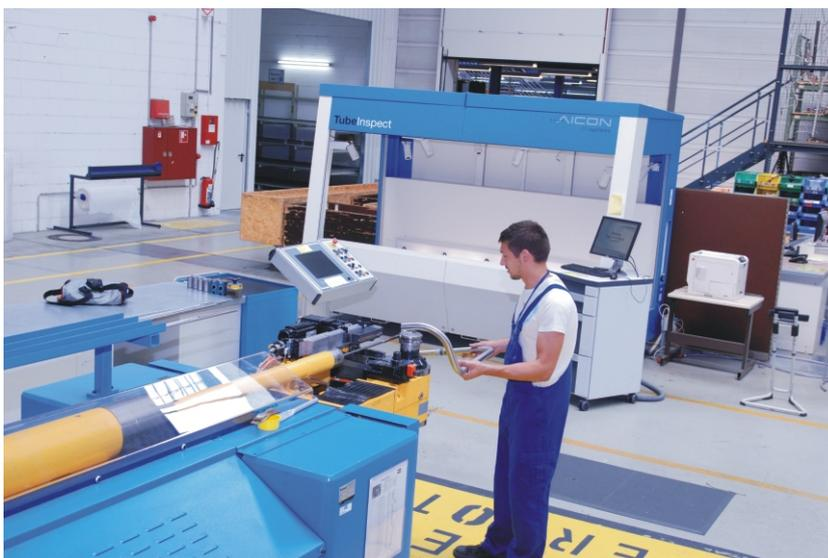
◉ Tube bending machine applied at PFW Aerospace
