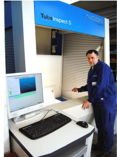
Valentin Medvedkins: “Thanks to TubelInspect, readjustment of our CNC bending machines is done instantly.”
